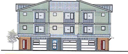
4 Front Roof Type 1 Front Elevation - Front Roof Alternate 3.02' x 11.0' Note: 1. Front bumpout adds 8 R2 per floor, per unit. 2. See Site Plan for applicable Front Roof Type 3. Building Type B2 shown.
