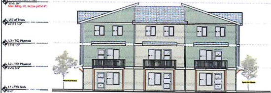
7 Rear Elevation - C1 3.02' x 11.0' Material Separation - Rear Exposing Face = 100.0 m 2 Unprotected Openings (Actual) = 47.4 m 2 (47%) Unprotected Openings (Allowed) = ≤ 30% Limiting Distance = ≥ 4.66 m (block 12)
