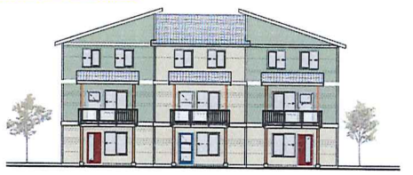
9 Rear Elevation - Street Facing Alternate - C4 3.02' x 11.0' Note: 1. Applies to Blocks 26 & 27, Building Type C4 shown. 2. Refer to Site Plan for applicable colour scheme
